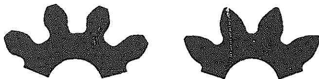
Figure 4. Left, a 10-tooth pinion with undercut resulting from pressure angle of 14½°; right, without undercut because of a larger pressure angle.
