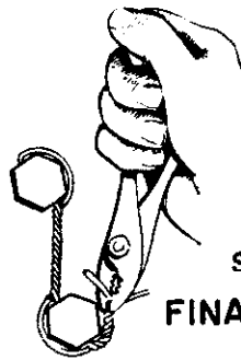
Figure 32. Standard twist safety wire installation procedure.
