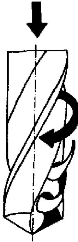
Figure 11 – Operation of drilling
