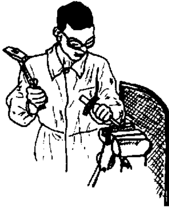
Figure 13 – Chiselling in front of the safety lattice
