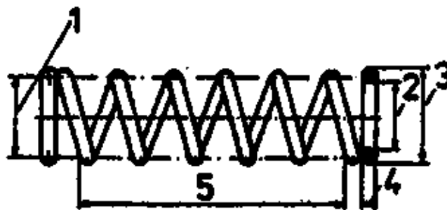
Figure 60 Compression spring 1 medium spring diameter D_m , 2 internal spring diameter D_i , 3 external spring diameter, 4 spring wire diameter D , 5 length of active coils
