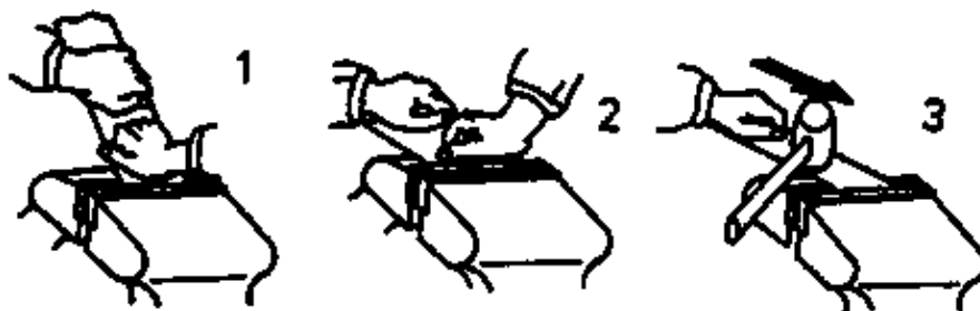
Figure 24 Bending of thin, long sheet metals 1 pre-bending by hand, 2 pre-bending with intermediate plates, 3 finish bending with a hammer
