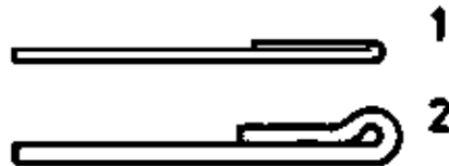
Figure 34 Turning up 1 thin sheet, 2 thick sheet
