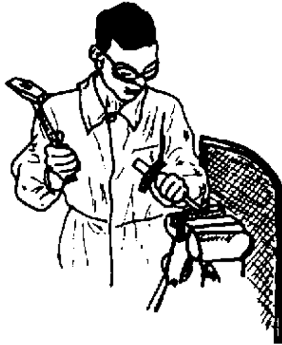
Figure 13 – Chiselling in front of the safety lattice
