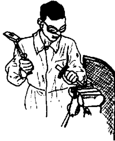
Figure 13 - Chiselling in front of the safety lattice
