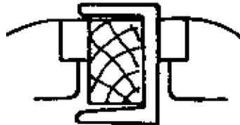
Figure 22 Wooden attachment for clamping of profiles
