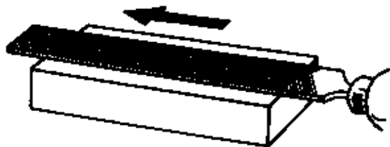
Figure 33 Longitudinal stroke filing
