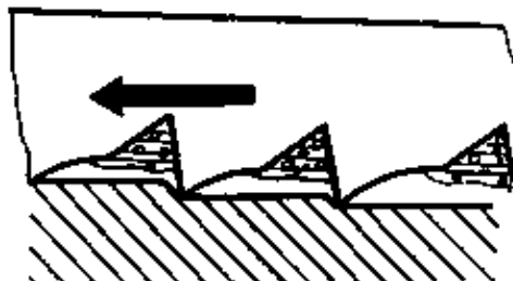
Figure 25 Chalked chiseled file
