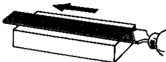
Figure 33 Longitudinal stroke filing
