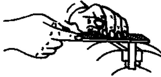
Figure 30 Handling of small files
