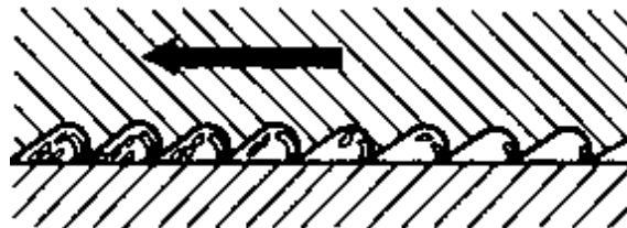
Figure 23 Action of the milled file
