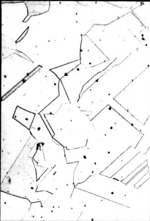
Etching bringing out grain boundaries in relief
