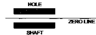
SIMPLIFIED SCHEMATIC DIAGRAM OF CLEARANCE FIT
