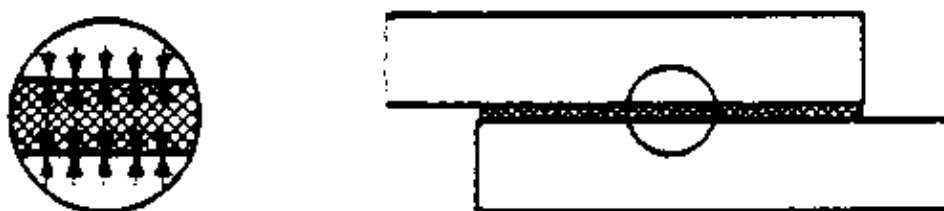
Figure 2/55 Specific adhesion of the adhesive
