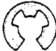
c) locking ring for shafts and axles
