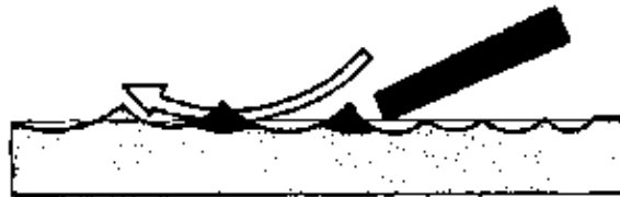
Figure 3/85 Principle of spot scraping
