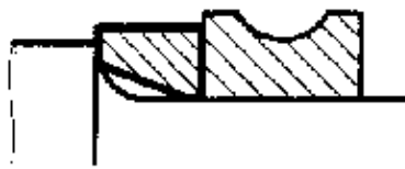
a) when the transition radius of the journal is too large,
