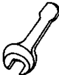
a) Single open-ended spanner with striking head;
