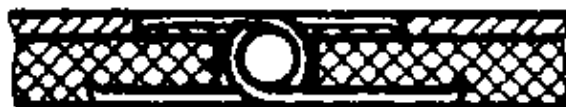
e Hook fastener for textile belts (sew butt leather on the ends of the belts to prevent fabric fraying)
