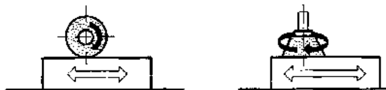
a Straight back and forth during flat grinding
