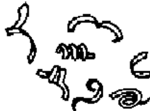
d Discontinuous chip
