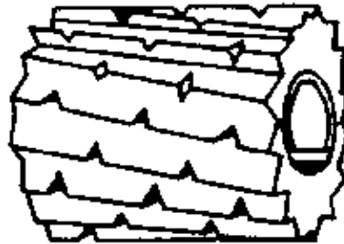
Figure 2.2.24. Milling cutter with chip-breaking grooves
