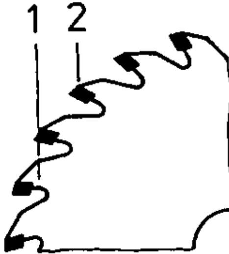
Figure 5.2.84. Circular saw blade with cemented carbide tips
