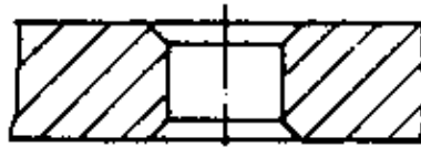
Figure 6.1.4. Drilling and countersinking the core diameter
