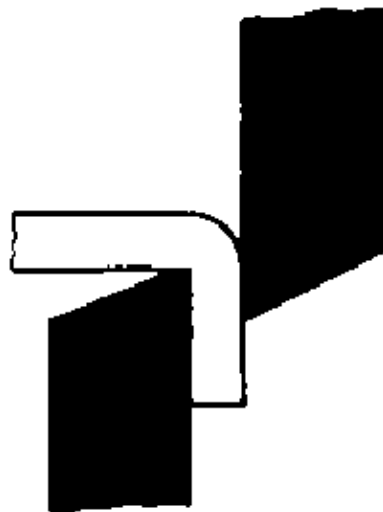
Fig. 2.2/9) Workpiece bent due to too large a cutting gap
