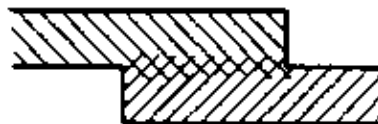
Fig. 4.3/14 Correctly soldered joint; the solder has penetrated into the surface of the metal parts
