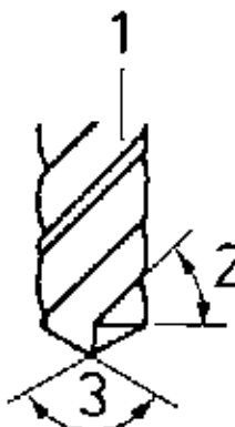
c) Drill type W for aluminium, tin, lead
