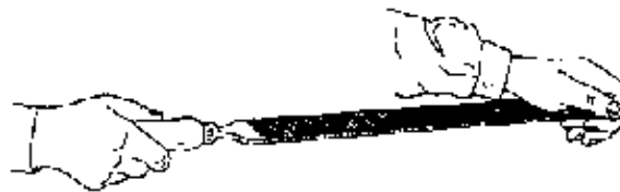
Fig. 2.4/16 How to guide a large file
