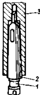
Fig. 2.5/9 Inserting a drill with drill socket
