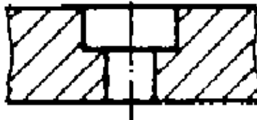
Fig. 2.6/1 Counterbore for filister head screw
