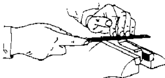
Fig. 2.4/18 How to guide a small file
