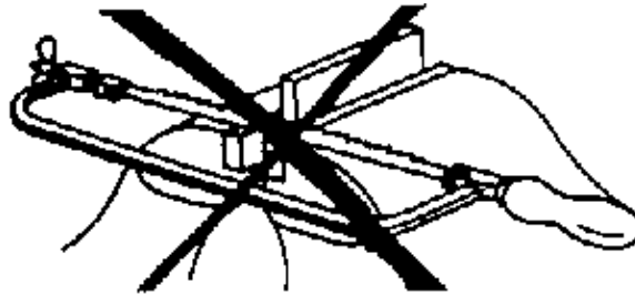
Fig. 2.3/15 Wrong! Do not saw along the vice jaws!
