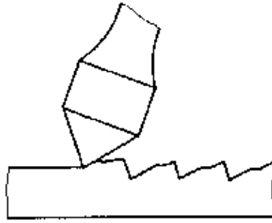
Fig. 2.4/2a Cutting of the file teeth with a special chisel; This results in notches and elevations which form together the file tooth.
