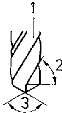
b) Drill type N for steel, cast iron
