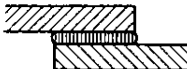
Fig. 4.3/15 "Dry soldered joint"; this joint has no strength and will loosen with the slightest load
