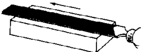
Fig. 2.4/26 Finishing in longitudinal stroke
