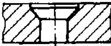
Fig. 2.6/7 Countersink for countersunk screw
