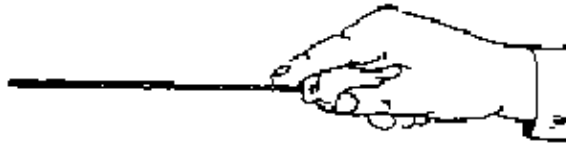
Fig. 2.4/19 How to guide a needle file (smallest type of files, cf. page ...)
