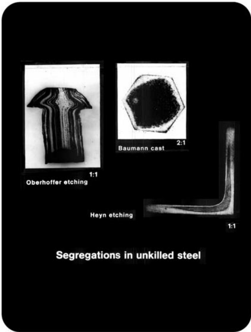
Film no. 10. Segregations in rimmed steel
