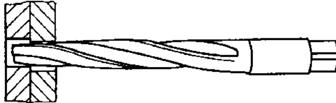
Figure 23 - Reaming of misaligned bore holes
