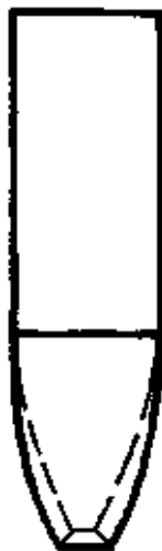
Figure 2. Grooving tool for special shapes
