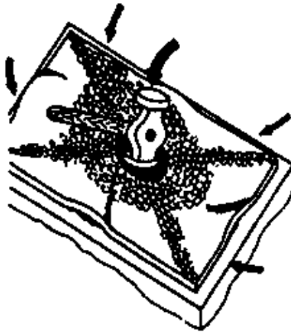
Figure 29 Straightening of a corrugated metal sheet by means of the straightening hammer
