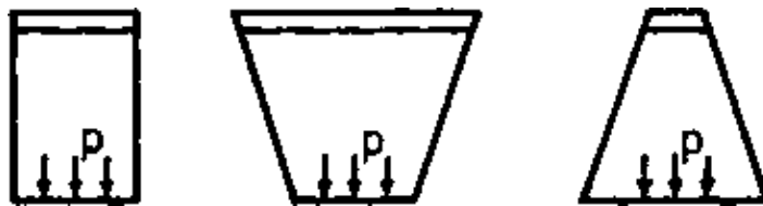
Fig. 7.5. The ground pressure is equally large in all three vessels.
