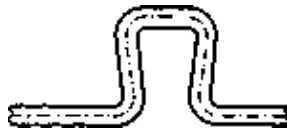
Fig. 6.18. Pipe expansion bends prevent damage to pipings, which convey liquids at highly differing temperatures.
