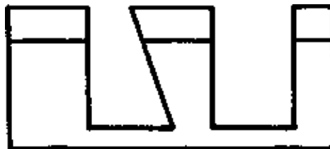
Fig. 7.1. In connected vessels, the liquid level is equally high.
