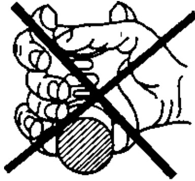
Fig. 2/77 Wrong application of the external limit gauge
