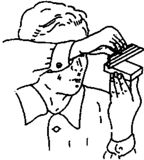
b – Testing is made according to light slit method at eye-level.
