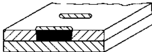
Plug weld: plug or slot weld/ USA
