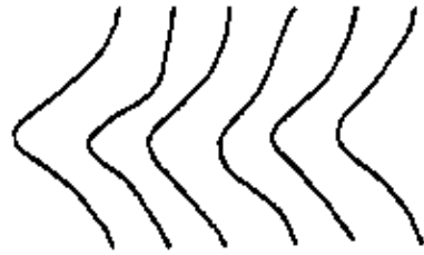
1 poor appearance of the bead ripples
