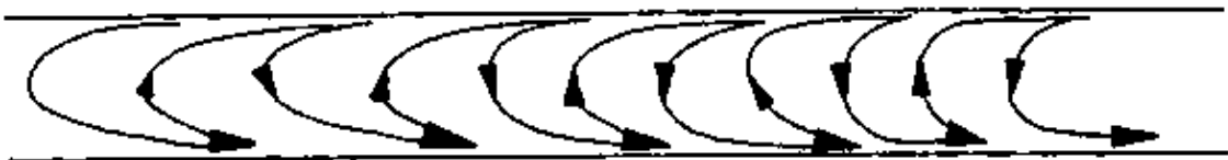
Fig. 18 a) Moving the electrode for the root welding
