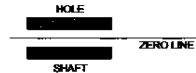
SIMPLIFIED SCHEMATIC DIAGRAM OF CLEARANCE FIT
