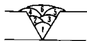
WELD BEAD PLACEMENT FOR MULTI-PASS BUTT WELD
