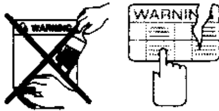
Replace unreadable labels
