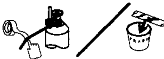
Repair or replace cracked gas hose
