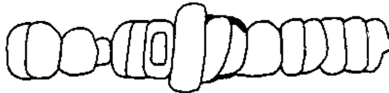
2 Welded bead with weld defects
