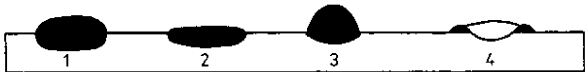
2 Welded bead with weld defects
