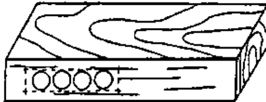
Figure 11 – Single bores to fill the long hole
