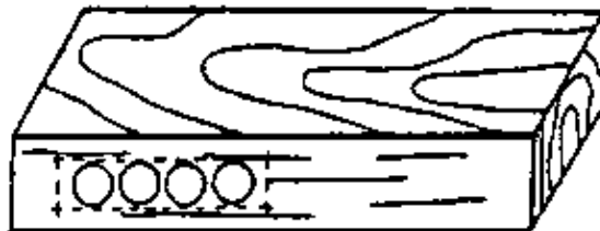
Figure 11 – Single bores to fill the long hole
