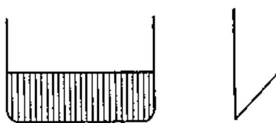
Figure 11 Rounding of edge corners at the plane iron
