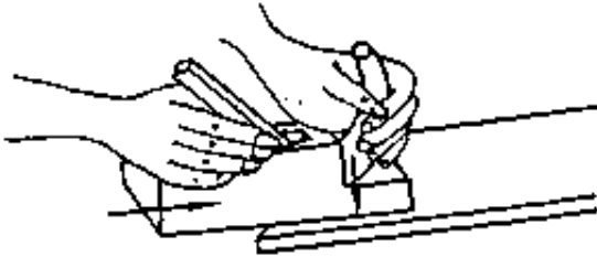
Figure 18 Applying the plane (starting of planing)
