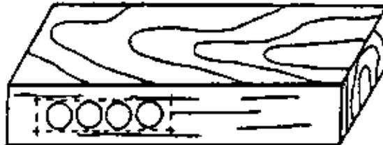
**Figure 11** – Single bores to fill the long hole
