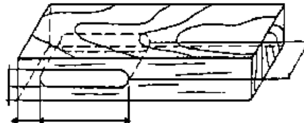
Figure 13 - Checking the long hole
