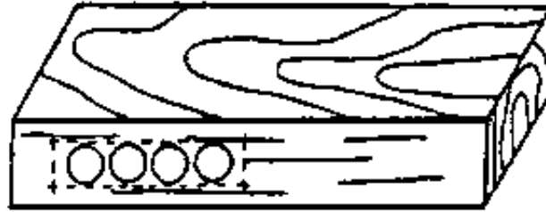
Figure 11 - Single bores to fill the long hole
