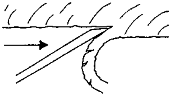
Figure 8 – Principle of veneer production
