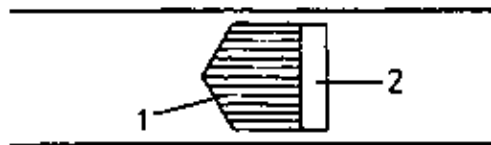
Figure 12 Insertion of a piece of hardwood into the plane face
