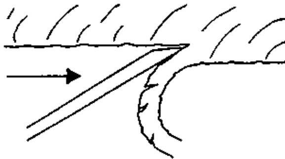
Figure 8 – Principle of veneer production
