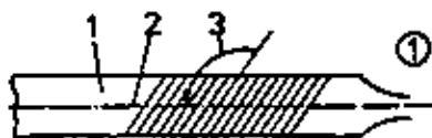
Figure 3 Types of files according to the cut rows, angles of cut rows (1) Single-cut file
