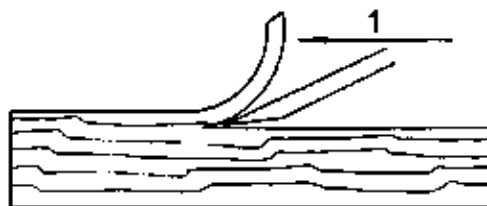
Figure 10 Correct cutting direction
