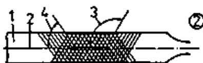
Figure 3 Types of files according to the cut rows, angles of cut rows (2) Double-cut file
