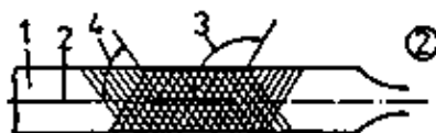
Figure 3 Types of files according to the cut rows, angles of cut rows (2) Double-cut file
