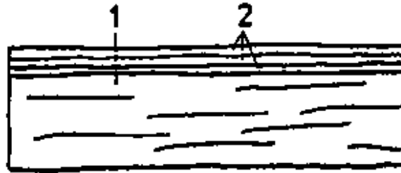
Figure 18 Making up process 1 board, 2 varnish layers individually applied
