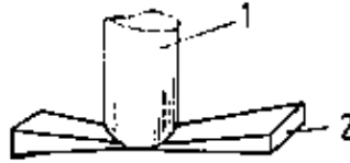
Figure 6 Column foot with wedge support
