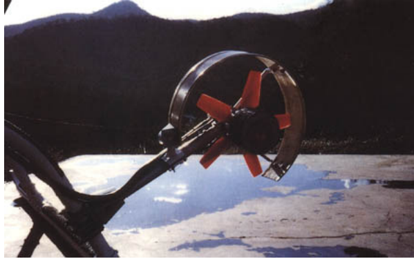
Plate 9. A metal or fibre glass shroud protects the fuselage should blades break off during flight.
