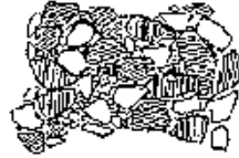
Fig. 4.9: Bad soil structure
