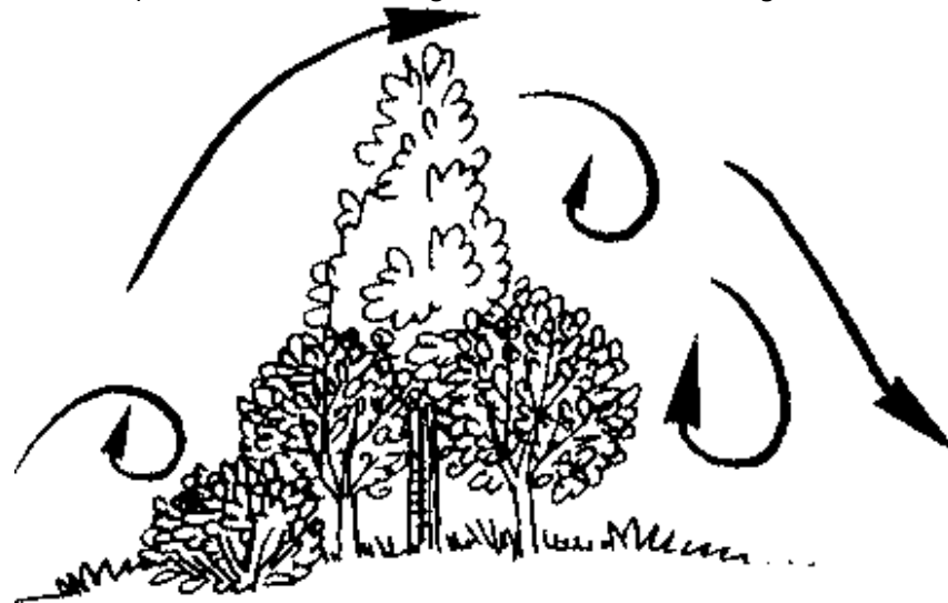
shelterbelt too dense - causes turbulence
