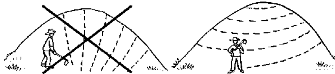
Work along the contour lines
