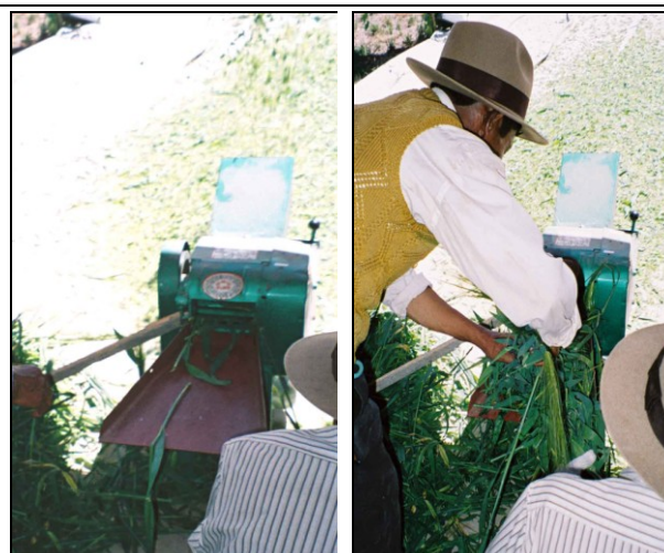
9.2.3. Wedge feed rolls part open to feed soft fodder
