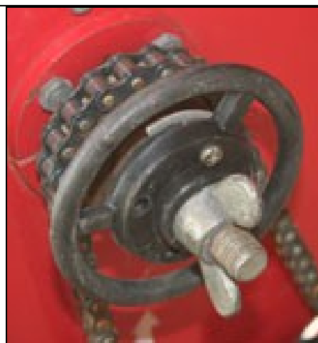
Plate 6B.13. Seed or fertilizer adjustment wheel and lock nut
