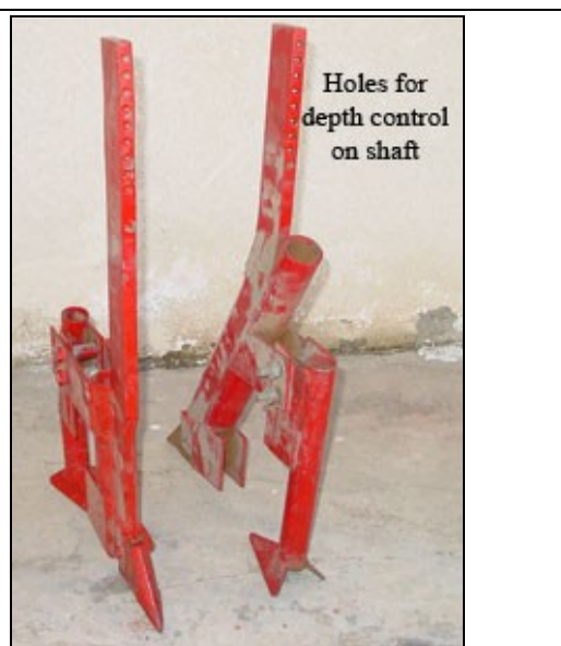
Plate 6B.4. Shaft of the opener that is raised or lowered to adjust depth of planting.
