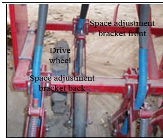
Plate 6B.5. Space openers by loosening and moving the brackets to get desired distance between rows
