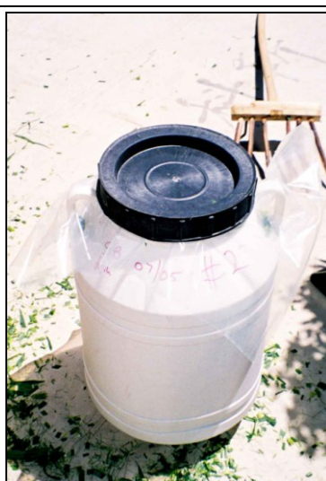
9.3.4. Seal with thick plastic sheet, inner plastic lid and screw cover
