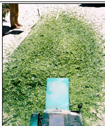
9.2.4. Chop fodder for two barrels at one time - note crop fractionisation
