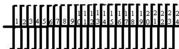
Figure 6A.4. Rotary blade installation for full cutting coverage (normal tillage)
