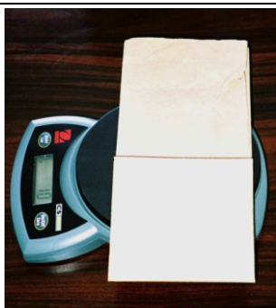
9.4.3. Tare balance for empty bag, and weigh fresh samples to 1g
