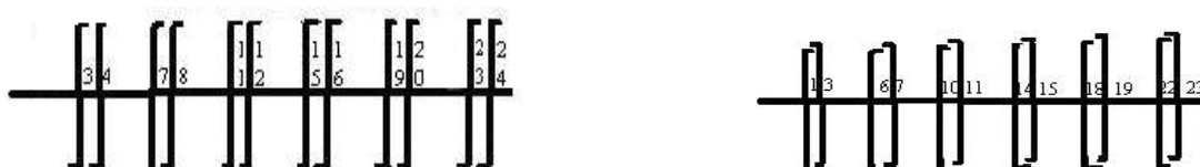
Figure 6A.5 Power tiller seed drill blades to give 15 cm tilled strips (on left) and 10 cm tilled strips (on right)
