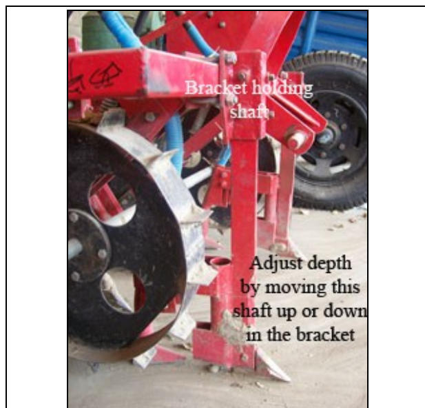
Plate 6B.4. Shaft of the opener that is raised or lowered to adjust depth of planting.
