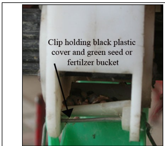
Plate 6B.9. Clip holding plastic cover and the plastic cover
