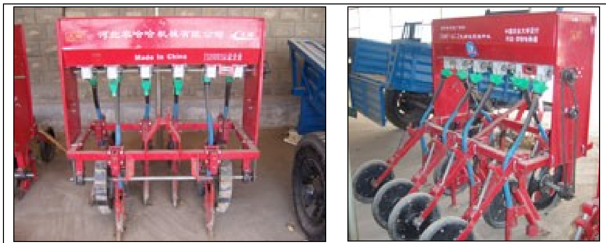
Plate 6B.1. Zero-till drill from the front and side, set up for 6 rows – 4 in the rear and two in the front; and for seed (front) and fertilizer (back box).
