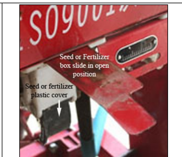
Plate 6B.8. Seed and fertilizer slide and plastic cover shown open
