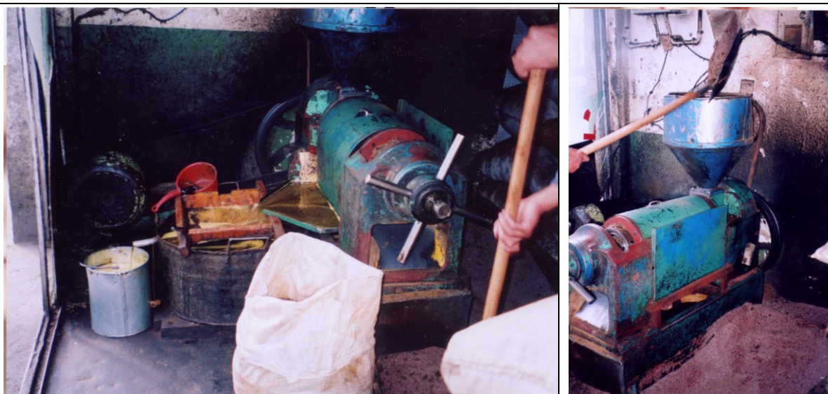
7.17.2. Family run oilseed mill in Lhasa city. Purchased rapeseed is being milled, passed through the mill three times. Oil is coarsely filtered to the left of the mill; rapeseed meal/cake is bagged off from the front of the mill after the third pressing.
