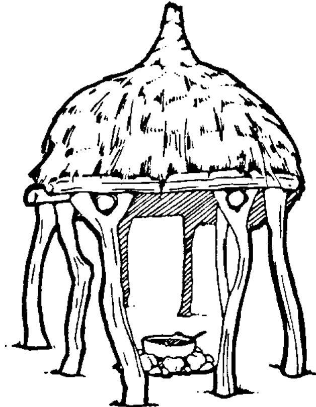
Fig. 7 Traditional dryer/storage in attic of cookhouse, Kenya
