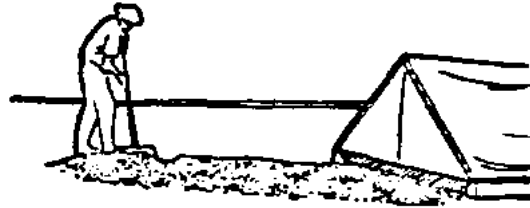
Fig. 14 Concrete drying floor with foul weather cover, Columbia
