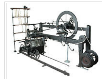
The only surviving example of a Spinning Mule built by the inventor Samuel Crompton
