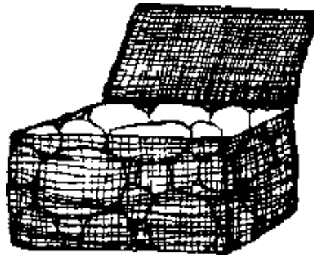
Figure 8-8. Gabion filled with stone, lid open
