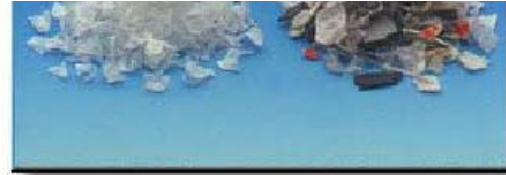
Fig. 11: Mixed and colour sorted PET-chips (flakes) after shredding, washing and fine separation
