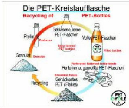
Fig. 13: Recycling cycle of PET-bottle waste to new bottles
