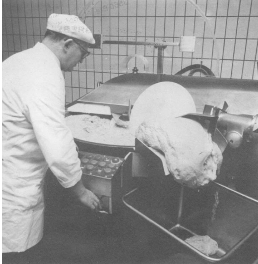
Fig. 9 THE CUTTER EQUIPPED WITH DEVICE FOR EMPTYING IT
