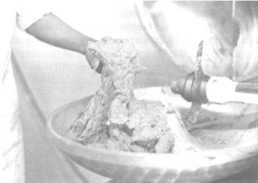
Fig. 33 THE MEAT EMULSION IS FORMED WHEN THE PROTEINS ARE SOLUBILIZED AND THE FAT PARTICLES SUSPENDED AND ENTRAPPED WITHIN THE PROTEIN MATRIX. THE FINISHED EMULSION IS TRANSFERRED TO A STUFFER
