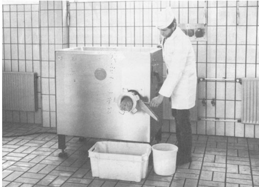
Fig. 6 GRINDER (Winkelwolf 130 mm) EQUIPPED WITH A DEVICE FOR SEPARATING THE CARTILAGE, TENDONS AND BONE PARTICLES FROM MUSCLE TISSUE (Photo courtesy of Kraemer und Grebe, GmbH & Co KG, D-3560 Biedenkopf-Wallau, W.Germany)
